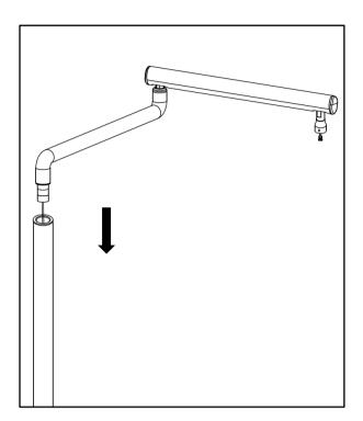
4. Pass the lamp shaft through the cosmetic ring and connect the wires, make sure the lamp shaft is well inserted into the level arm, fully fasten with one M5\*12 screw.
