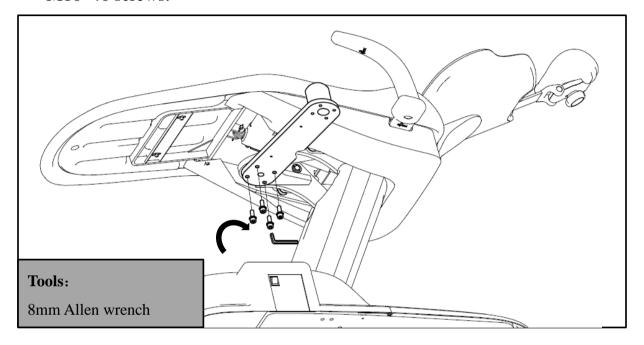
2. Insert the intermediate post into the installing hole on the fixing plate, assure the verticality through a levelling instrument, and finally fasten the post by four M8\*10 screws.
