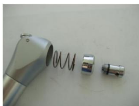
Figure 1 Angled Syringe Tip Locking Retainer Uninstallation
