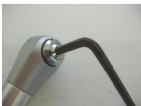
Figure 1 Angled Syringe Tip Locking Retainer Uninstallation
